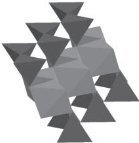
FIGURE 5. Stoichiometric Periodic Bond Chains (PBCs) for a dioctahedral 2:1 phyllosilicate. (a) Chain running parallel to the (110) face. The ( \bar{1}10 ) face is symmetrically equivalent. (b) Chain running parallel to the (010) face.
